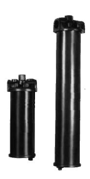
The 1B1 and 1B2 Model Cartridge Filter Housings, three-piece housings featuring center post construction, offer a choice of either cast iron an steel or 304 stainless steel as the materials of construction. The 1B1 and 1B2 Model Cartridge Filter Housings have flow rates of up to 16 GPM, and accept working pressures and temperatures up to 175 psig at 250°F. The 1B1 and 1B2 Model Cartridge Filter Housings are available as one- or two-high cartridge models.
